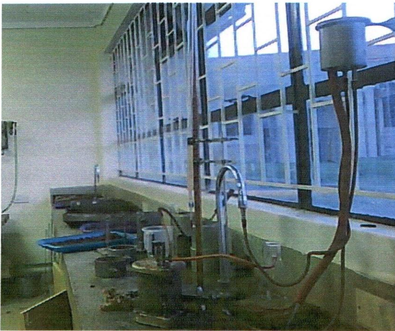
Plate 5: Constant head permeability test arrangement
