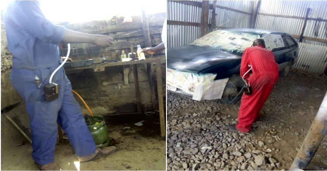
Plate 3.5: Task based airborne sample collection for radiator repairs and spray painting
